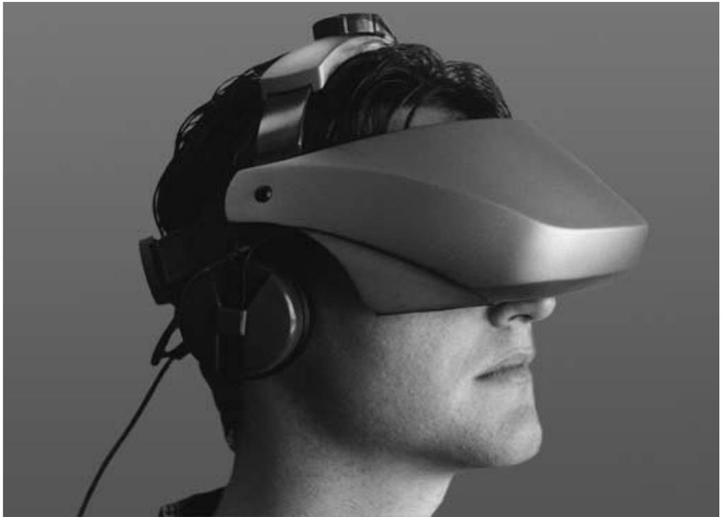
Figure 4: HMD 800-35 (Source: Image courtesy of Fifth Dimension Technologies)
