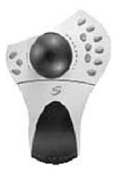
Figure 1: Spaceball 4000 FLX (Source: Image courtesy of Labtree)
